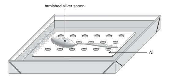
On a silver spoon, the black tarnish,  $Ag_2S$ , can be removed spontaneously by placing the spoon in contact with aluminum in a conducting solution.
