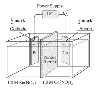
a) Label the anode and cathode in the space provided on the diagram above. (1 mark)
